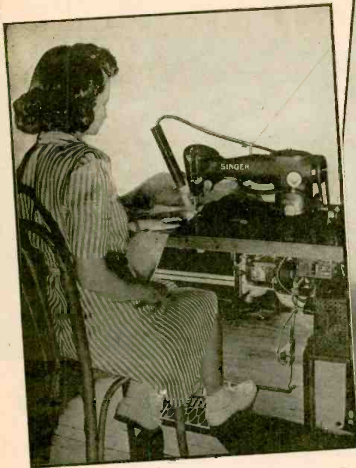
Left: a standard machine fitted with the electronic guard. Right: a closer view of the details of the "seeing-eye" device.
